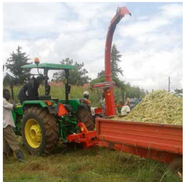
Forage harvester harvesting maize for silage making in one of the farms
